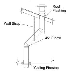
Figure 30 - Offset with Wall Strap and 45° **Elbows**
